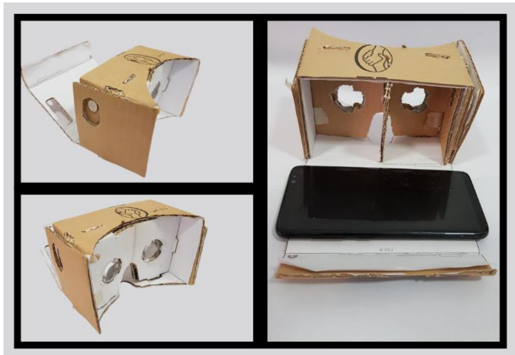
Figure 5: Google Cardboard display assembled for the experiment, according to the specifications in (Google C, 2023), and shown in figure 3.
