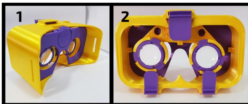
Figure 7: Prototype assembled after FDM printing. 1: rear view; 2: front view.
