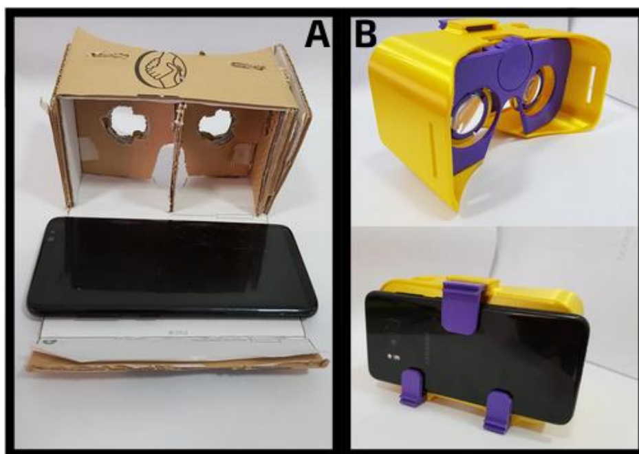
Figure 10: Displays produced during the study side by side. A: cardboard model; B: FDM printed model.
