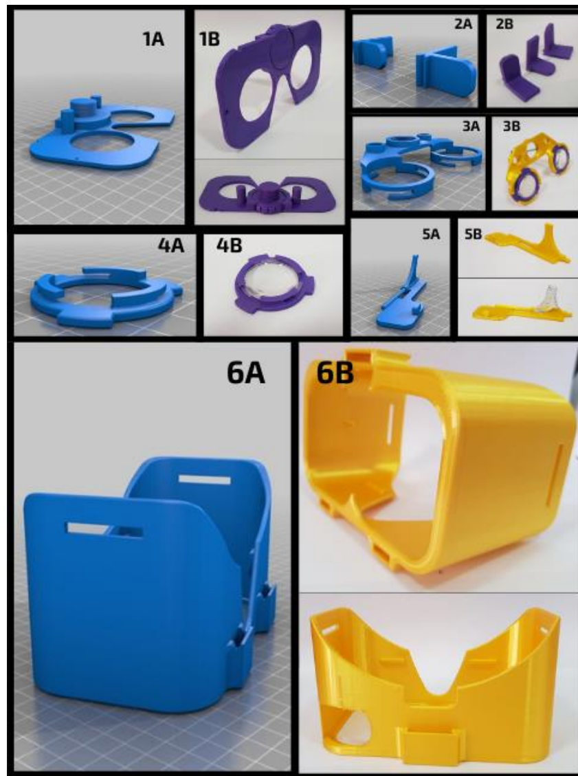
Figure 6: Digital model of the prototype and its FDM printed equivalent. 1: Lens holder; 2: Smartphone holder; 3: Lens base; 4: Lens adapter; 5: Button; and 6: Body.
